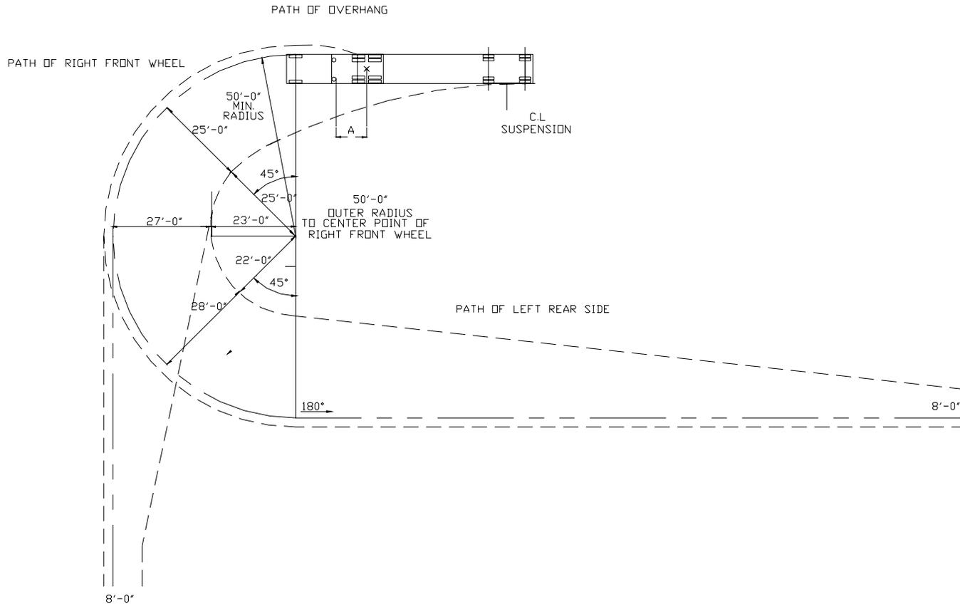
**Figure 7: Turning Requirements**
