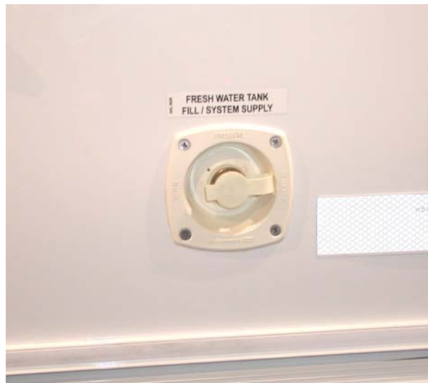
Figure 17: Fresh Water Tank Fill
