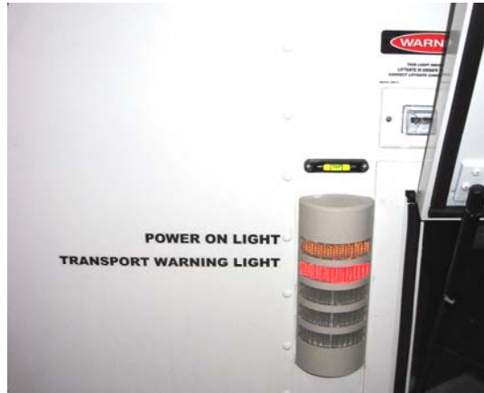
AC Power ON Light and Platform lift Transport Warning Light
