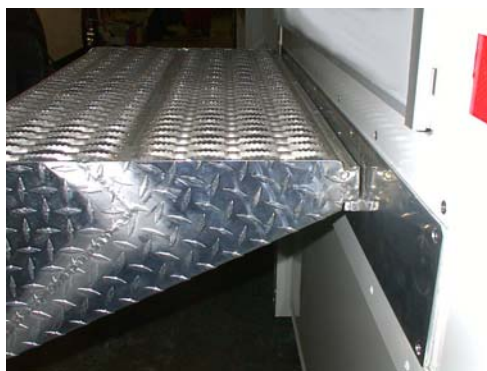
Figure 21: Stair Assembly (standard)
