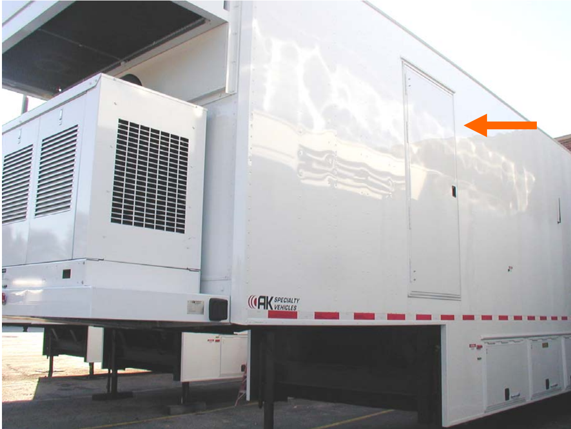
Figure 24: Emergency Exit / Service Door
