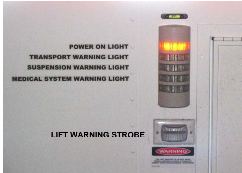
Figure 50: Lift Transport Warning Strobe
