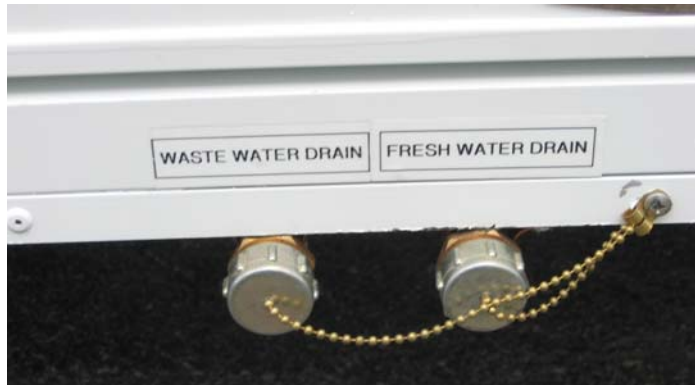
Figure 31: Fresh & Waste Water Drain Connections
