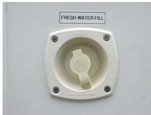
Figure 30: Fresh Water Connection
