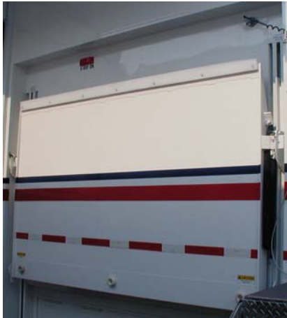
Lift Stored for Transport
